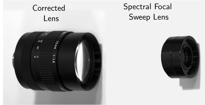
Figure 3.2: A comparison showing the relative sizes and complexities of a Cosmimar 75mm F/1.4 lens (left) and our F/4 SFS doublet lens (right). Our lens is significantly lighter and more compact. The corrected lens is stopped down to F/4 in all experiments.
