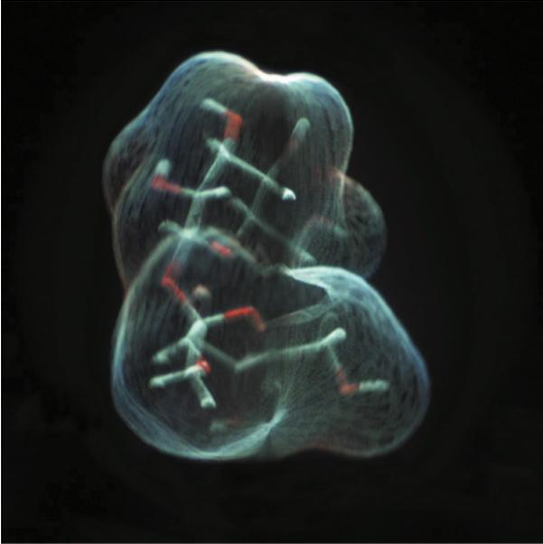
Fig. 3. (Color online) Photograph of a sugar molecule as reconstructed by the Perspecta multiplanar volumetric display before modification. The molecule's inner structure is visible through the necessarily translucent outer shell.
