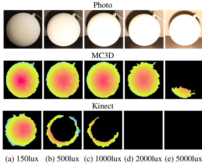
**Fig. 2:** Output Under Ambient Illumination. Disparity output for both methods captured with 1 second exposure at 128x128 resolution (Kinect output cropped to match) under increasing illumination from 150 lux to 5000 lux measured at middle of the sphere surface. The illuminance from our projector pattern was measured at 150lux. Note that in addition to outperforming the Kinect, MC3D returns usable data at ambient illuminance levels an order of magnitude higher than the projector power.
