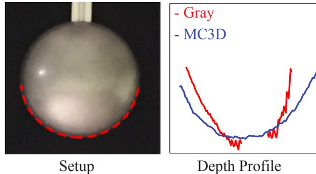
**Fig. 4** : Performance with Reflective Surfaces. The image on the left depicts a reflective test scene consisting of a shiny steel sphere. The plot on the right shows the depth output from Gray coding and MC3D. Both scans were captured with an exposure time of 1/30th second. The Gray coding method used 22 consecutive coded frames, while MC3D results were averaged over 22 frames. The Gray code output produces significant artifacts not present in MC3D output.
