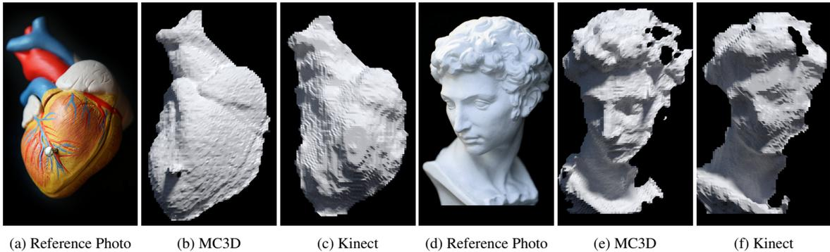
**Fig. 1:** Comparison between Motion Contrast 3D Scanning (MC3D) and Microsoft Kinect. Kinect and MC3D methods captured with 1 second exposure at 128x128 resolution (Kinect output cropped to match) and median filtered. Object placed 1m from sensor under 150 lux ambient illuminance measured at object.
