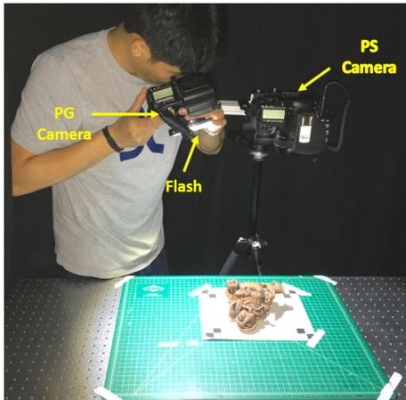
Fig. 2: **capture setup:** We use two Canon 5D Mark III cameras with 50mm prime lens. The PS camera is placed about 0.5m away from the object.
