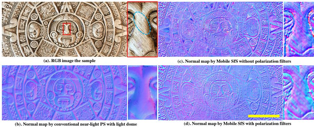
Fig. 6. **Surface normal for the plaster replica of an Aztec calendar stone:** (a). the photo of the imaged sample; (b). the surface normal generated with near-light PS using light dome; (c). the surface normal generated using mobile SFS but without polarizers; (d). the surface normal reconstructed with the proposed mobile SFS. Close-up images shows the "nose" on the plate. Scale bar: 5 cm.
