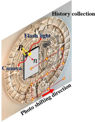
Fig. 4. **Acquisition procedure with Mobile SfS:** Hand-held Mobile SfS faces to the object. Slightly shift the phone and take one image at each position. Nine images are taken in this paper for the surface normal reconstruction.
