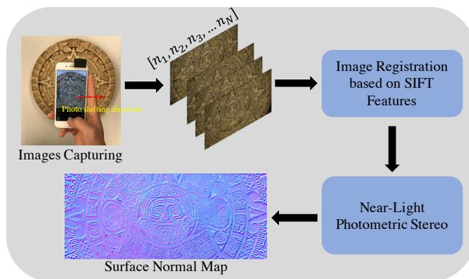
Fig. 1. **Overview of Shape from Shifting:** Our shape-from-shifting technique uses a mobile device camera to capture images around the object with the built-in flash used as a source of illumination. SIFT-based image registration renders the images to the same viewpoint but each with a unique illumination direction. The synthesized images are further processed by uncalibrated photometric stereo to acquire dense surface normal vector maps.
