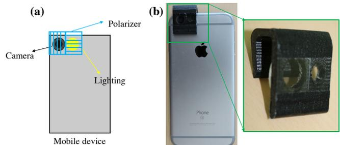
Fig. 2. **Mobile Sfs hardware:** (a). two polarizers with opposite polarization are attached to the camera and the flash light of the mobile device, respectively; (b). photo of our prototype Mobile Sfs with an iPhone 6 and a custom 3D printed widget.
