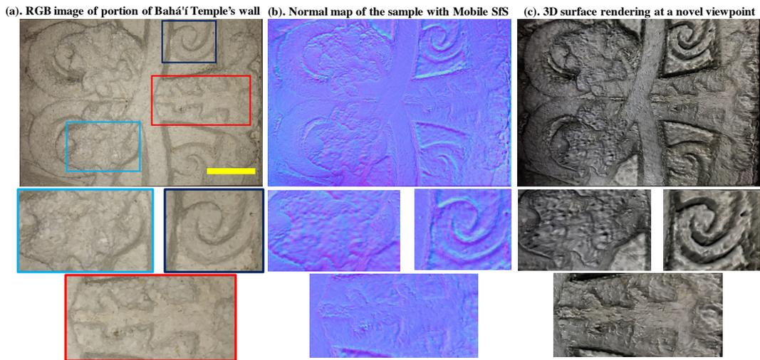
Fig. 7. **Surface normal for the architectural elements:** (a). photo of the region of Bahá'í Temple which is been scanned; (b). the surface normal generated with mobile SFS; (c). the rendering with surface normal generated with mobile SFS. Close-up shows the detailed feature on the stone. Scale bar: 10 cm.
