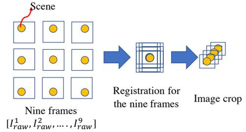
Fig. 5. **Image pre-processing:** Step 1: nine images are captured; Step 2: images are registered with the SIFT function; Step 3: images are cropped to display the same region.
